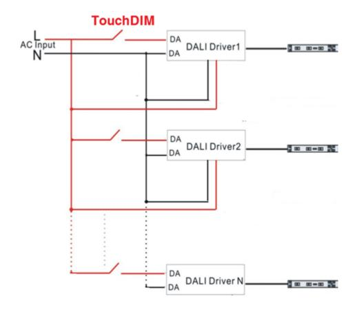
**Remark:** Only use open push button without indicator light. Maximum cable length between each Unit: 20 meters.
